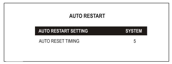
The source qualification timer dictates how long to allow for input and bypass voltages to return to their nominal limits. The default value is 100 with a programmable range of 5-100 minutes. Since a setting of 100 signifies an infinite wait time, the finite range can be set between 5 and 99 minutes. Normally, 5 minutes is adequate.
